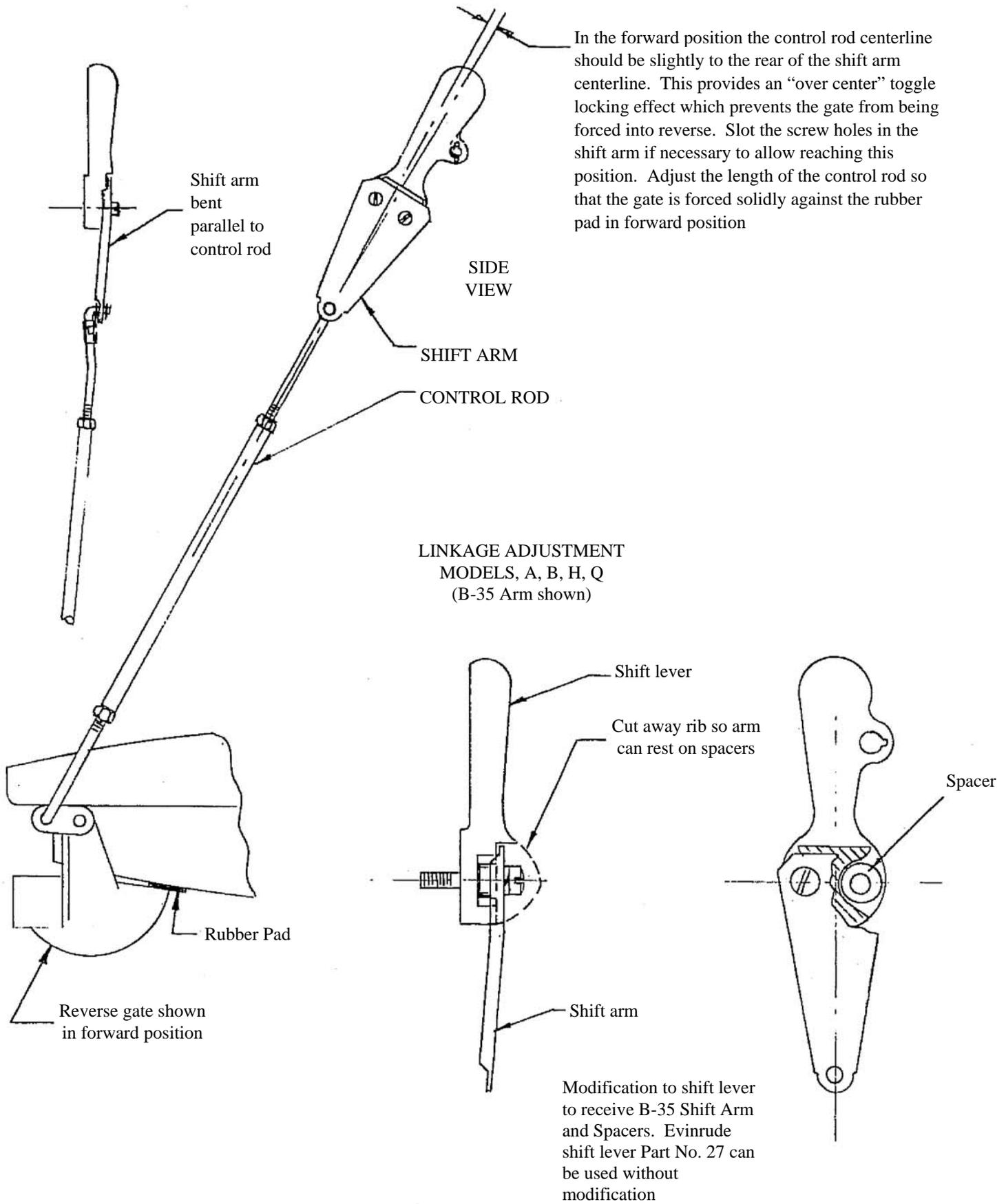
Modification to shift lever to receive B-35 Shift Arm and Spacers. Evinrude shift lever Part No. 27 can be used without modification
