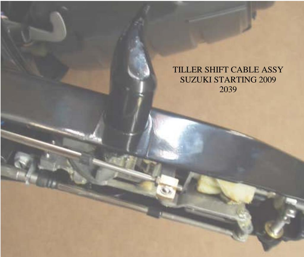
1. Remove the lower plastic cover from the steering handle.
