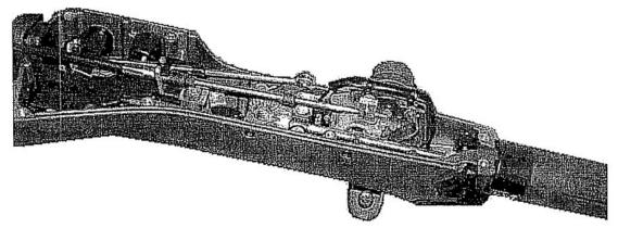
1. Remove the lower plastic cover from the steering handle.
